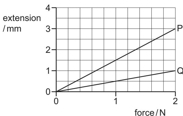
The wires have the same original length but different diameters.
