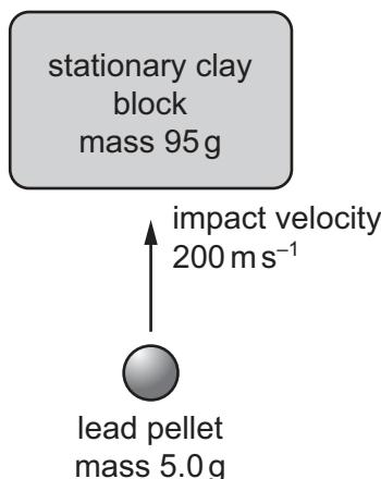
The mass of the pellet is 5.0 g and the mass of the clay block is 95 g.
