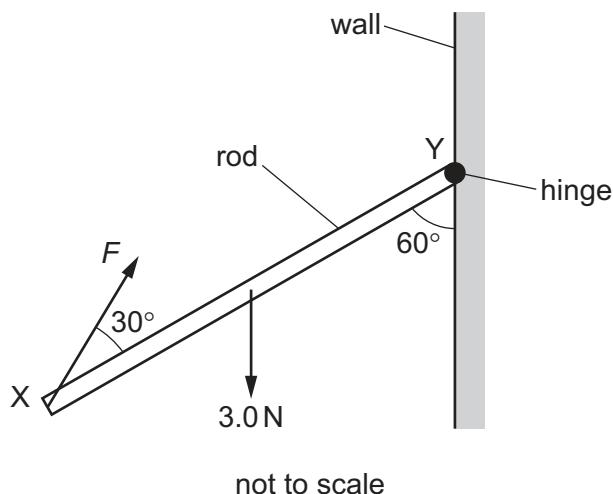
A force  $F$  acts at an angle of  $30^\circ$  to the rod at end X. The rod has a weight of  $3.0\text{ N}$  and is in equilibrium.
